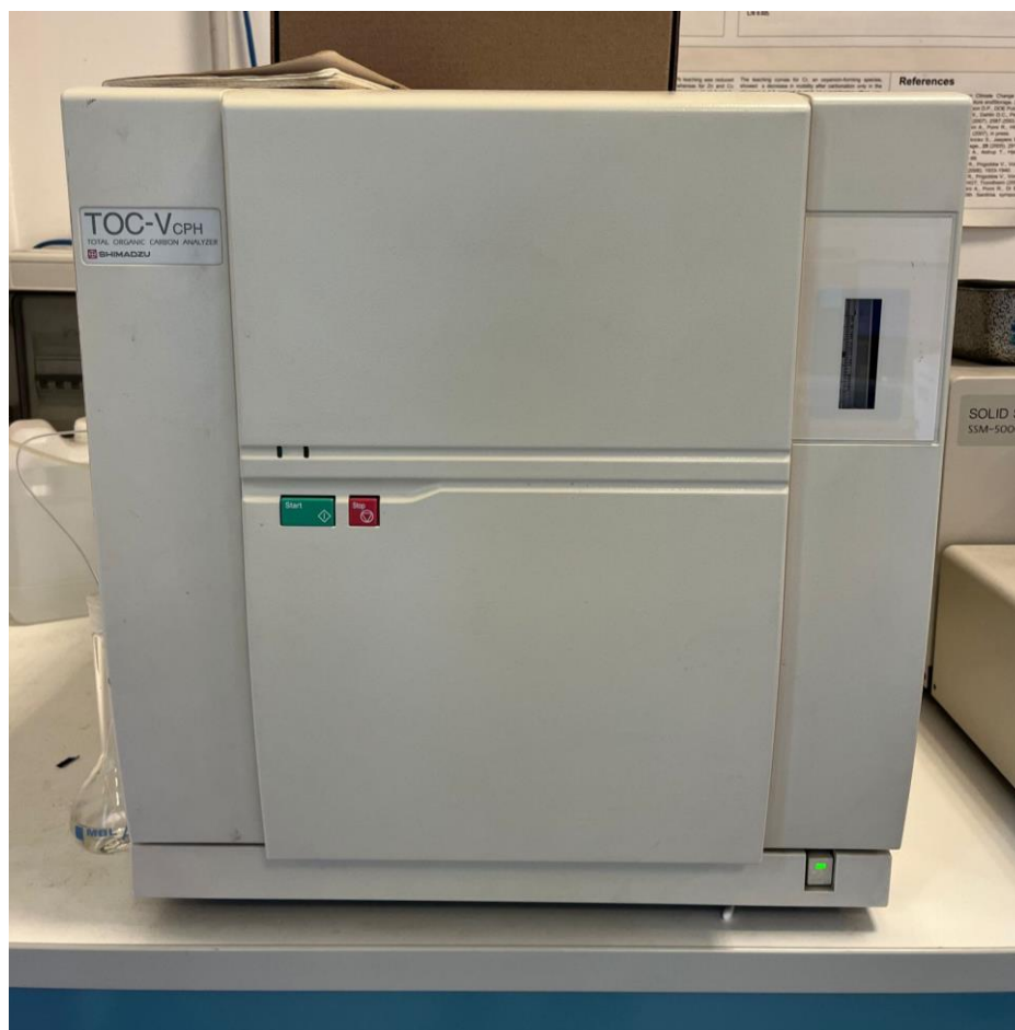
Figure 14. Total organic carbon analyzer from Shimadzu
