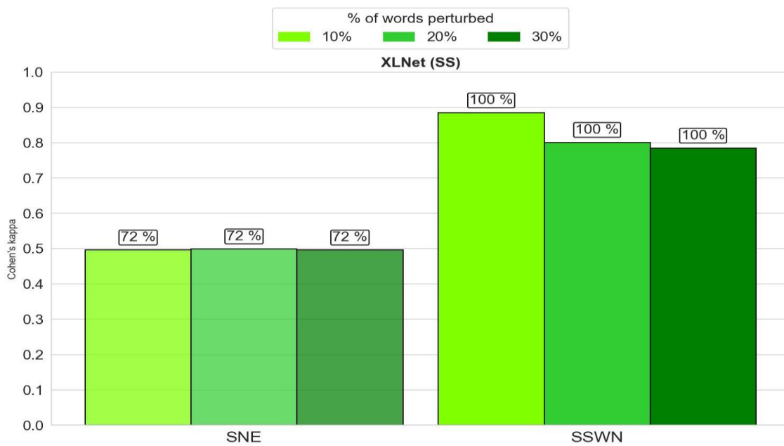
Figure 47. Cohen's kappa values for word level perturbations per perturbation percentage using XLNet in the Semantic Similarity task. The values above the bars show the proportion of perturbed samples for that given perturbation
