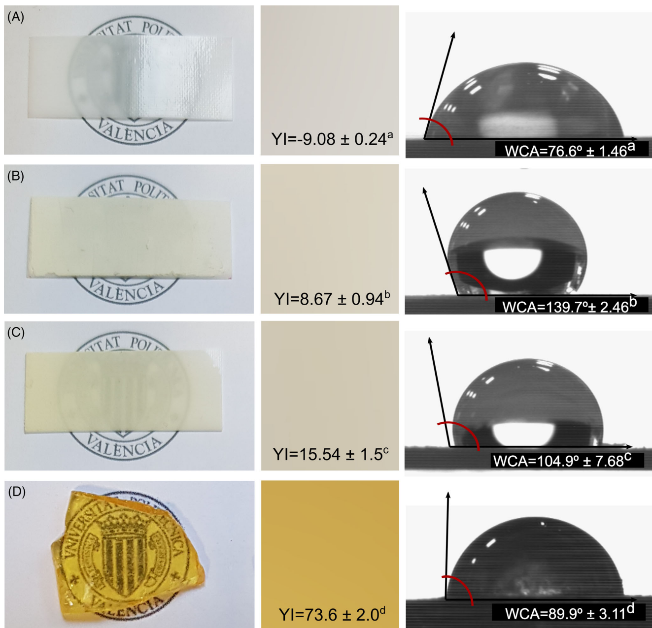
FIGURE 3 Visual appearance, yellowness index, and water contact angle of (A) PCL, (B) PCL-eGRDCM, (C) PCL-eGRCF films, and (D) neat GR. Different letters (a–d) show statistically significant differences between formulations ( p < 0.05 )
