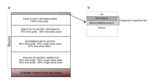
**Figure 1.** (a) Stratigraphy of a typical stucco test tube. The square denotes the area enlarged in (b) that delimits the thin film studied in the present investigation formed on the surface of the *intonachino* (upper stucco layer).
