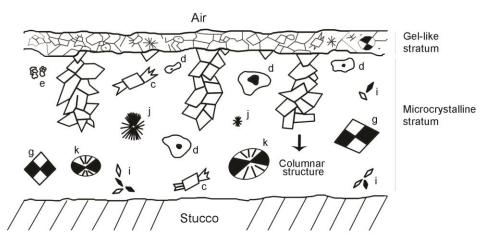
**Figure 3.** Sketch of the epigenetic superficial film in section. Letters correspond to the crystalline phases and other particles shown in Figure 2 (modified from [29]). Note that although the gellike stratum is mainly composed of sub-micron particles of calcium carbonate (*vide infra*), some of the crystallochemical phases identified in the microcrystalline stratum may be also present in the outermost layer. Letters correspond to crystalline specimens and other particles shown in Figure 2.
