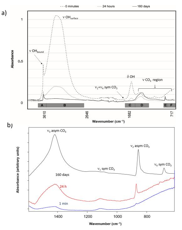
**Figure 6.** (a) IR spectra of samples taken from the surface of test tubes initially, after 24 h and after 160 days; (b) Detail of the 1500–600 cm<sup>-1</sup> region for the IR spectra.
