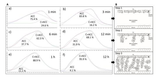
**Figure 7.** (A) Original overlapped band (blue line), sum band (red line) and individual bands of calcite plus ACC (C + ACC) (green line) and ACC (purple line) obtained by applying the mathematical curve-fitting process in the carbonate  $v_3$  stretching band at: (a) 1 min; (b) 3 min; (c) 6 min; (d) 1 h; (e) 1 h and (f) 12 h. Percentage values of the overlapped band area are provided. (B) Epigenetic superficial film at step 1 (0–3 min), step 2 (3–12 min) and step 3 (12 < time < 160 days).
