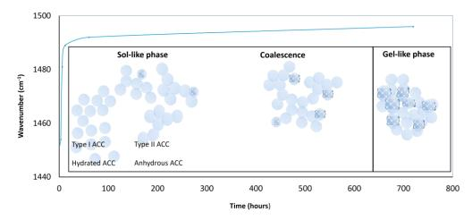
**Figure 12.** Maximum of the ACC band in the carbonate v stretch region versus time. Scheme of the presumed behavior of the ACC particles when forming the gel-like stratum in the epigenetic surface film.
