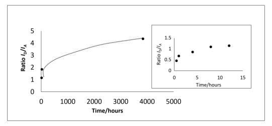
**Figure 9.** Diagram of the ratio of intensities of IR bands of calcium carbonate and calcium hydroxide  $(I_D/I_A)$  versus time. Insert shows in detail the 0–16 h interval.
