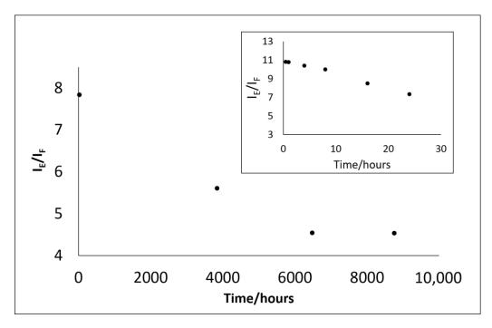
**Figure 10.** Diagram of the ratio of intensities of IR bands  $v_2$  and  $v_4$  of the carbonate group ( $I_E/I_F$ ) versus time. Insert shows in detail the 0–24 h interval.
