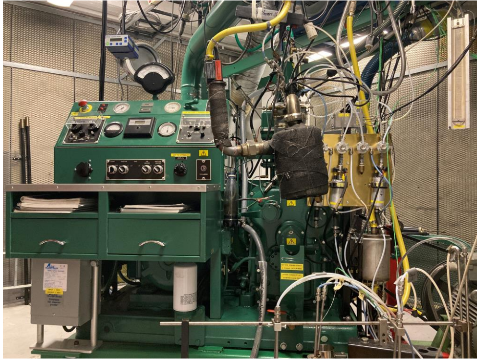
Fig.2. The modified CFR engine at the Energy sciences lab of Lund University.
