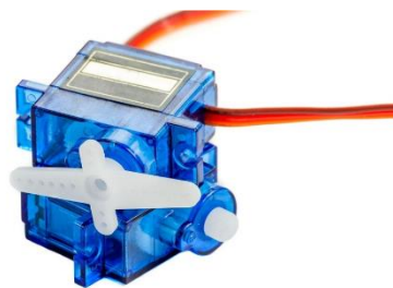
Figura 13: Servomotor a emplear modelo SG90 [9].
