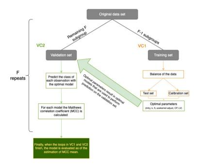
Figure 2.1: Diagram of the double cross validation used to evaluate the classification models.
