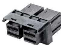
Figure 1.5.2: MiniSAS connectors to transfer data from the Digitizer to the DPB
