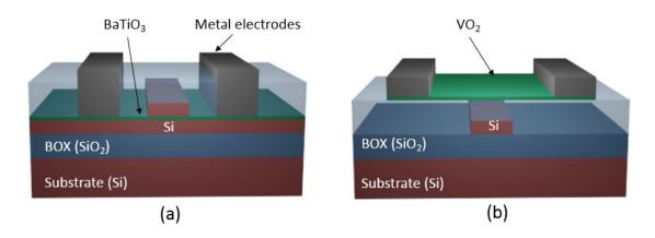
Fig. 2. Examples of Si-compatible (a) BaTiO<sub>3</sub> and (b) VO<sub>2</sub> waveguides.
