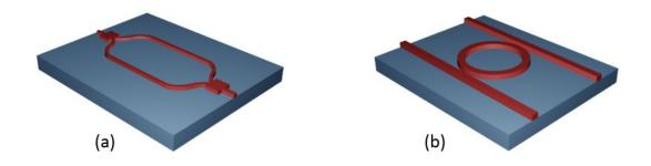
Fig. 1. (a) Mach-Zehnder interferometer and (b) ring resonator photonic structures.
