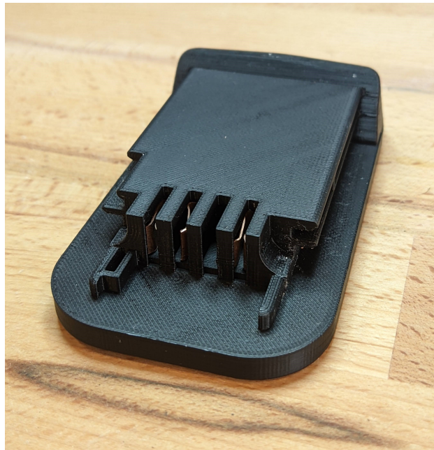
Figure 45: Battery Connector final version with metal connectors
