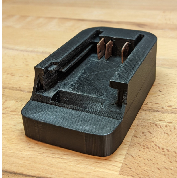
Figure 46: Power tool Connector final version with metal connectors
