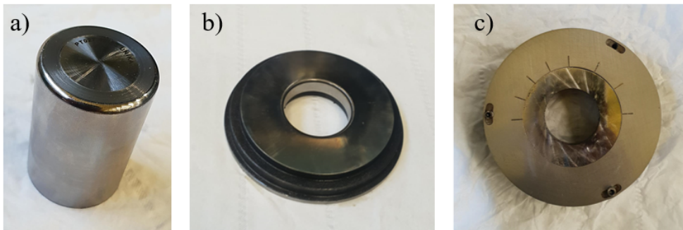
Figure 2.12. a) Deep drawing punch, b) deep drawing die, c) deep drawing blankholder.
