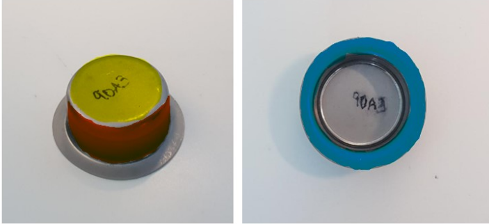
Figure 2.8. Cup with surfaces used for establishing base alignment. Blue: top plane of the flange, yellow: bottom plane, and red: outer walls surfaces.
