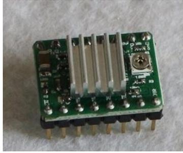
Figura 28. Stepper driver Pololu A4988 (Tienda Prometec Spain, 2022b).
