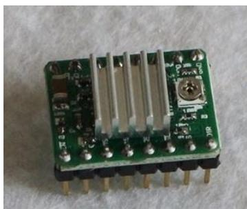
Figura 124. Stepper driver Pololu A4988 (Tienda Prometec Spain, 2022b).
