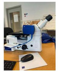
Figure 2.5: Zeiss Axio Zen 2 core machine
