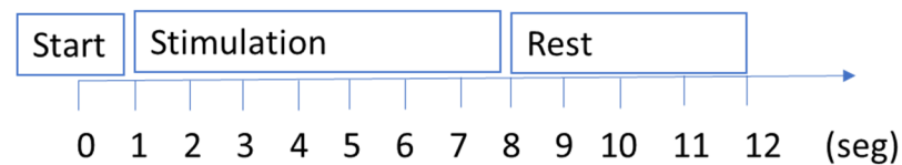
Figure 3. Timing of a single SSVEP trial.
