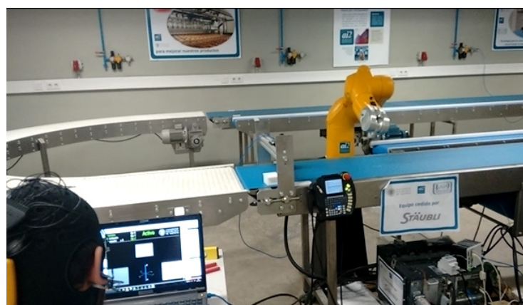
Figure 14. SSVEP BCI control of the Stäubli robotic arm.
