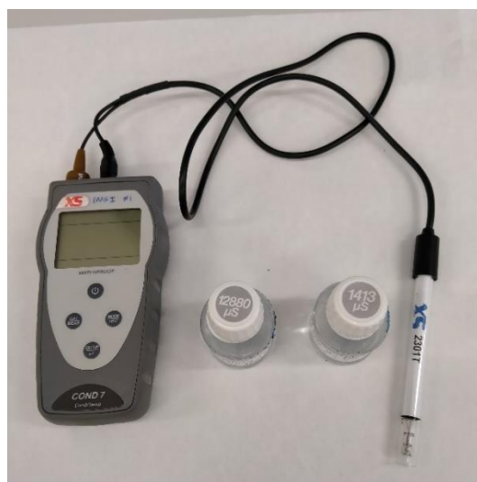
Figure 3. Conductivity meter with \pm 1\% full-scale accuracy.
