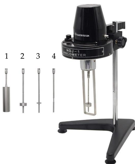
Figure 2. Rotational viscometer with needles numbered from 1 to 4.
