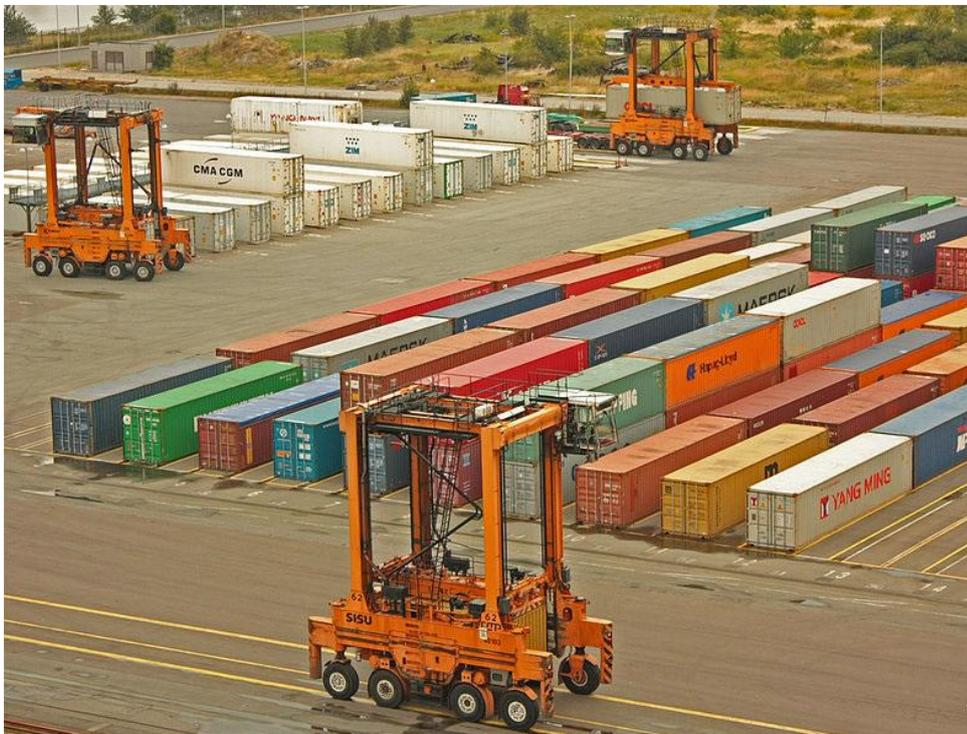
Figura 4 - Straddle Carrier. Fuente: (Endo f an era: The last Kalmar classic straddle Carrier leaves the factory, s.f.)
