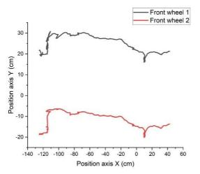
Fig. 7 X vs Y trajectory of the assistive device with the directional locking and anti-reverse systems activated
