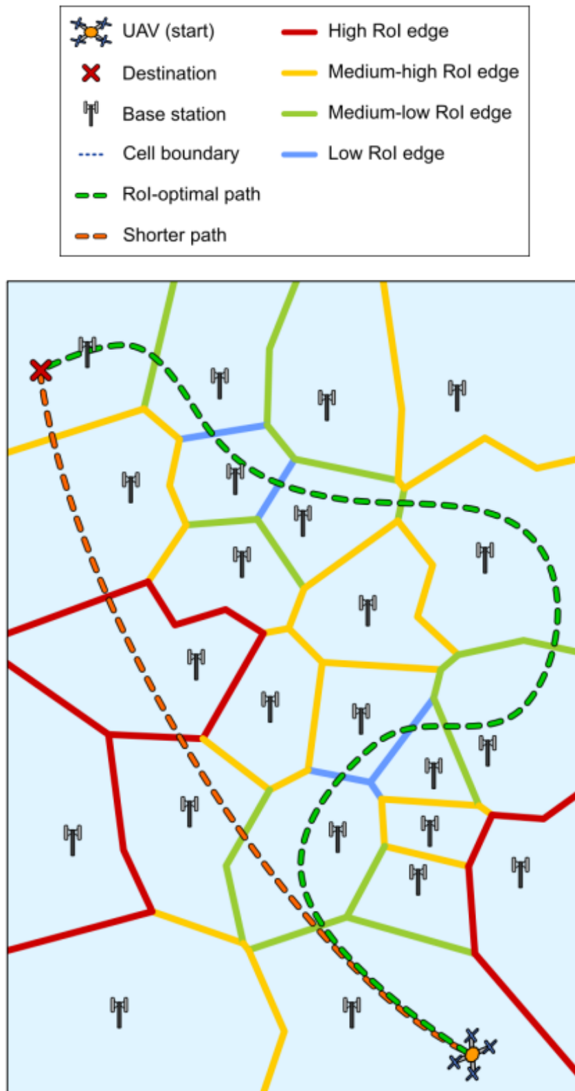
Figure 2.4: RoI-optimal path calculated compared to a possible shorter path.
