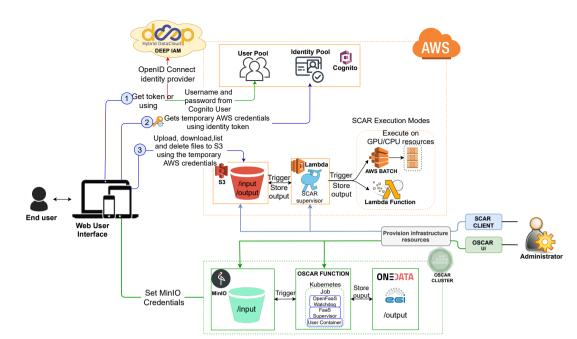
FIGURE 3 Architecture for the integration of Machine Learning models in AWS and an on-premises cloud.
