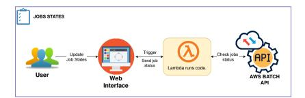
FIGURE 8 Check the status of jobs through a Lambda function.
