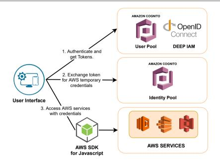
FIGURE 2 High-level authentication and authorization flow in the web interface.
