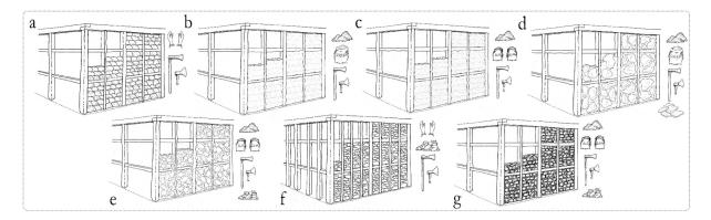
Figure 4. Classification of the different material variants with monolithic infills, from left to right: piled earth (a), *tapialete (b)*, lime and earth concrete (c), stone slabs in formwork (d), formwork masonry (e), stacked masonry (f) and ordinary masonry (g).
