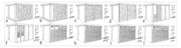
**Figure 6.** Classification of the different material variants with rigid screens, from left to right: open vertical laths (a), closed vertical laths (b), open horizontal laths (c), closed horizontal laths (d), simple lath-and-daub with earth (e), simple lath-and-daub with plant fibres (f), double lath-and-daub with earth (g), double lath-and-daub with earth and plant fibres (h), double lath-and-daub with stones (i), and double lath-and-daub with boards (j).
