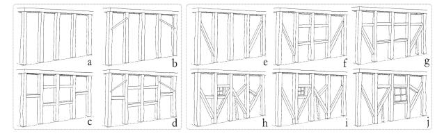
**Figure 3.** Classification of different geometric variants, from left to right: group of simple geometries (V (a), V with braces (b), V + H (c), V + H with braces (d)) and group of complex geometries (V + D (e), V + H + D (f), V + H + X (g), V + X (h), V + X + D (i), V + H + D + X (j)).
