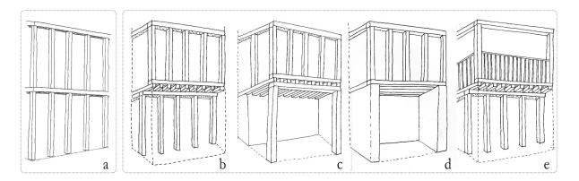
Figure 2. Classification of the different typological variations from left to right: continuous wall (a), projecting discontinuous wall (b), discontinuous wall in portico layout (c), and discontinuous wall in arcade layout (d), and discontinuous wall in gallery layout (e).
