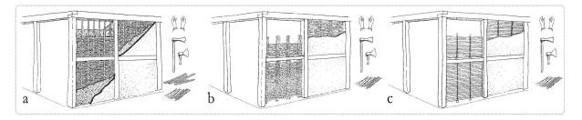
Figure 7. Classification of the different material variants with flexible screens, from left to right: wattle-and-daub (a), mesh (b) and reed structures (c).
