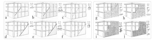
**Figure 8.** Classification of different rendering variants, from left to right: group of continuous renderings (earth on infill (a); lime and/or gypsum on infill (b); limewash on infill (c); completely earth (d); completely lime (e); completely limewashed (f)) and a group of discontinuous renderings (boards (g); slate slabs (h); convex and concave roof tiles (i); only convex roof tiles (j)).
