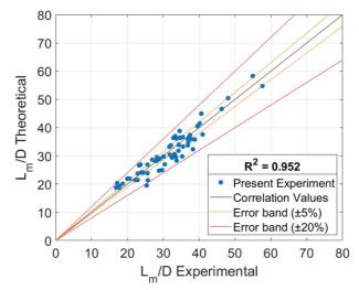
Figure 8: Comparison of calculated dimensionless momentum length and experimental measurements.
