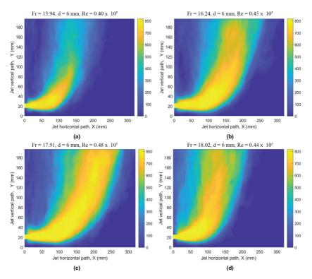
Figure 5: Experimental results for horizontal buoyant jets in stagnant water (a)  $V_a = 0.25$ , (b)  $V_a = 0.5$ , (c)  $V_a = 0.79$ , (d)  $V_a = 1$ .
