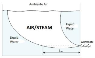
Figure 3: Behavior of a horizontal gas jet into liquid ambient.
