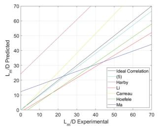
Figure 9: Trend of momentum length prediction values with respect to the nozzle diameter with different correlations.
