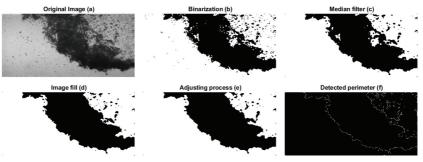
Figure 4: Routine realized in MATLAB to determine the jet interface.
