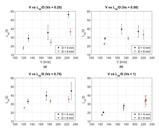
Figure 7: The influence of velocity on the momentum length (a)  $V_a = 0.25$ , (b)  $V_a = 0.5$ , (c)  $V_a = 0.79$ , (d)  $V_a = 1$ .
