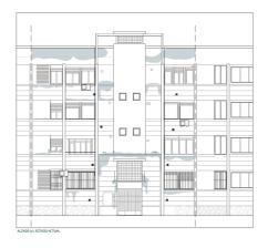
Figure 10. Example of the planimetric survey made of the previous and the current status. Pathologies and modifications are shown. Linear building
