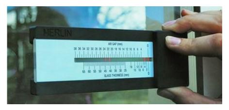
Figure 6. Glass thickness measure using Bohle, Merlin Laser device
