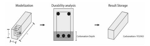
Figure 3. Steps for the durability analysis
