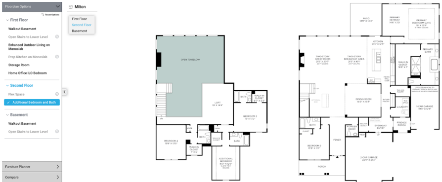
Figure 6. Toll Brothers "Milton" model, first and second floors plan; Located adjacent to an individual bedroom, the ensuite bathroom is arguably the precursor to the value and desires that have guided the internal formal and programmatic character of the single-family dwelling in the United States. In figures 4-6, the architectural proposal set in motion by the Gamble House, continues in the plans and construction of dwellings of non-architectural origins, as seen in the Toll Brother's house plan. The plan shows how millions of homes have been and continue to be constructed adhering to not only a planimetric and programmatic concept, but also reflects the values held by Americans today regarding their homes.
