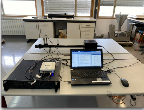
Figure 4.2 Impedance Tube measurement setup (left). Representative specimens of melamine and rockwool in 100mm and 38mm diameter (right)
