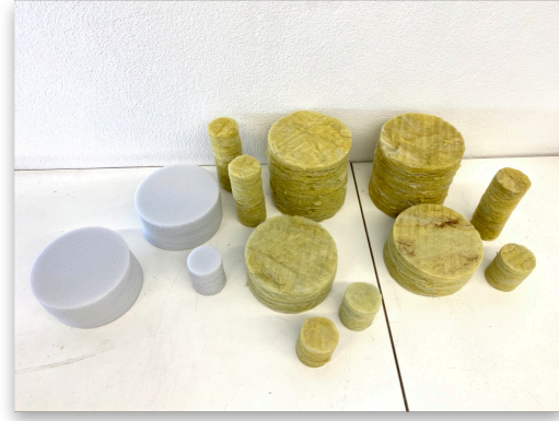
Figure 4.2 Impedance Tube measurement setup (left). Representative specimens of melamine and rockwool in 100mm and 38mm diameter (right)
