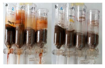
**Figure 4.** Percolation tubes of the soils amended with straw at the end of the incubation experiment in (**a**) flooded treatment; (**b**) non-flooded treatment.
