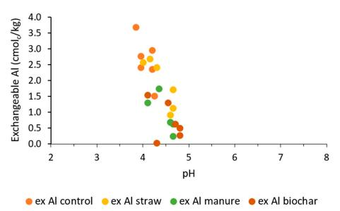
**Figure 11.** Relationship between soil pH and exchangeable aluminum in the soil at the end of the second incubation experiment.
