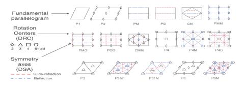
Fig. 2. Representation of the 17 Wallpaper Groups, their standard notation and their internal symmetries. The UL is referred as Fundamental Parallelogram.
