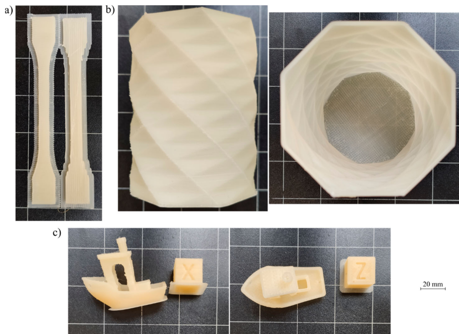
Figure 9. Examples of the PHBH 3D-printed parts: (a) dog bone samples with both infills; (b) pencil pot; (c) benchy and a calibration cube.
