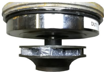
Fig. 6. Impeller of the wet-rotor pump with two clogged channels.
