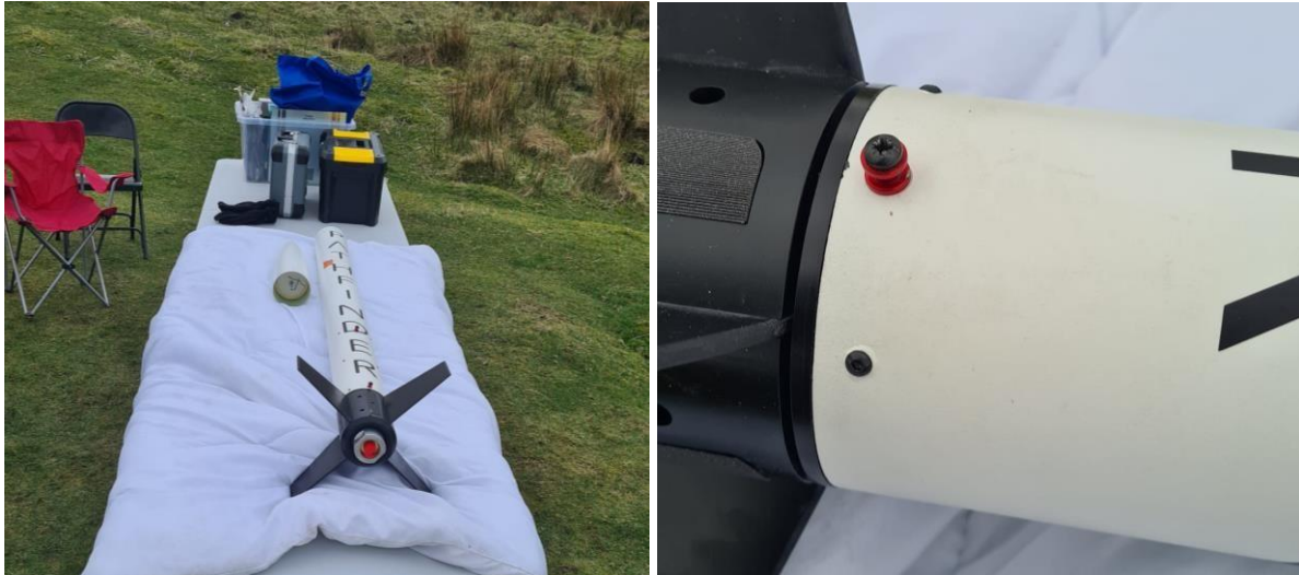
Figure 13: The rocket (left photo) and the red fixations for the rail (right photo)
