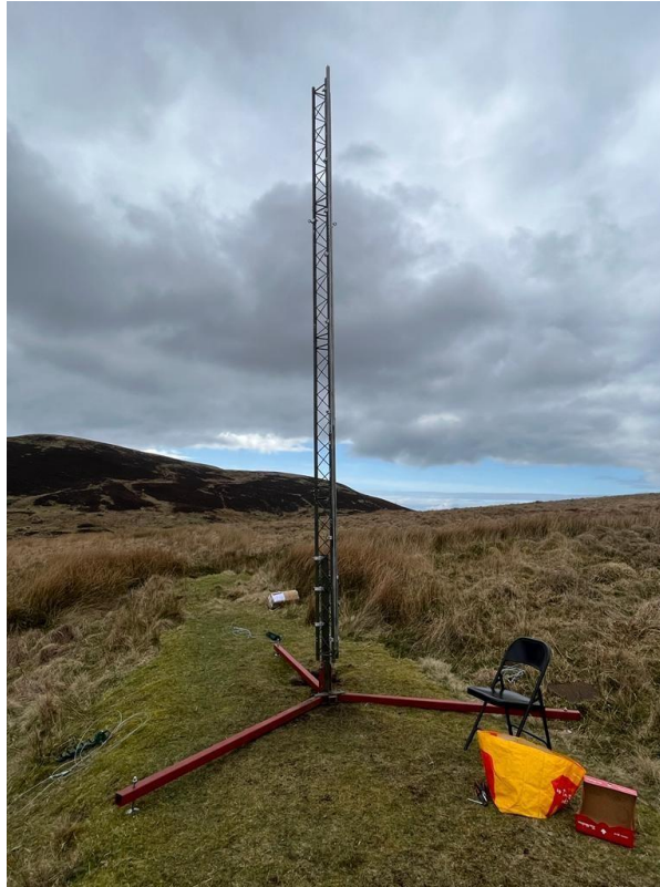
Figure 12: The launching rail fully assembled
