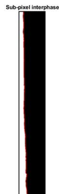
Figure 16. Result of the application of the subpixel detection algorithm to the grey image (layer edge in red color).
