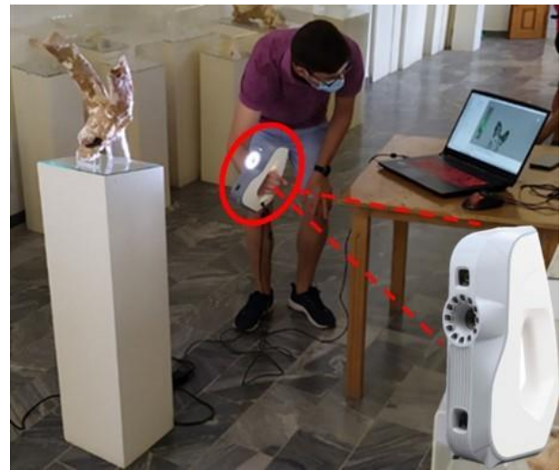
Figure 10: Palaeontological findings mounted on rigid stands and the ARTEC EVA 3D Scanner.
