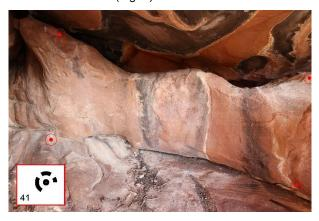
Figure 2: Location of the CPs (red dots) and sample image of the coded targets used inside the rock shelter.
