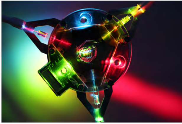
Fig. 1. LX assembly of three fiber arrays to a triangular shaped SiN PIC and a PCB for electrical interfacing. 45 degree on-chip mirrors are used to exit the visible light from the centre of the chip into free space.
