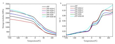
**Figure 5.** Comparative plots of the evolution of (**a**) storage modulus (E'), and (**b**) glass transition temperature ( $T_g$ ) as a function of the temperature of rPP pieces and the rPP/hemp fiber composites with different compatibilizers.
