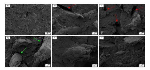
**Figure 2.** Field-emission scanning electron microscopy (FESEM) images of the fracture surfaces of the injection-molded rPP/hemp composite parts: (**a**) rPP; (**b**) rPP-H10-C; (**c**) rPP-H20-C; (**d**) rPP-H30; (**e**) rPP-H30-C; and (**f**) rPP-H30-M. Images were taken at 500×.
