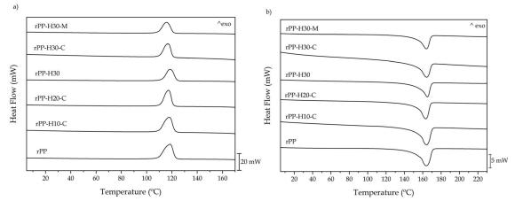
Figure 3. DSC thermograms of rPP/hemp fiber composites' (a) cooling cycle and (b) second heating cycle.
