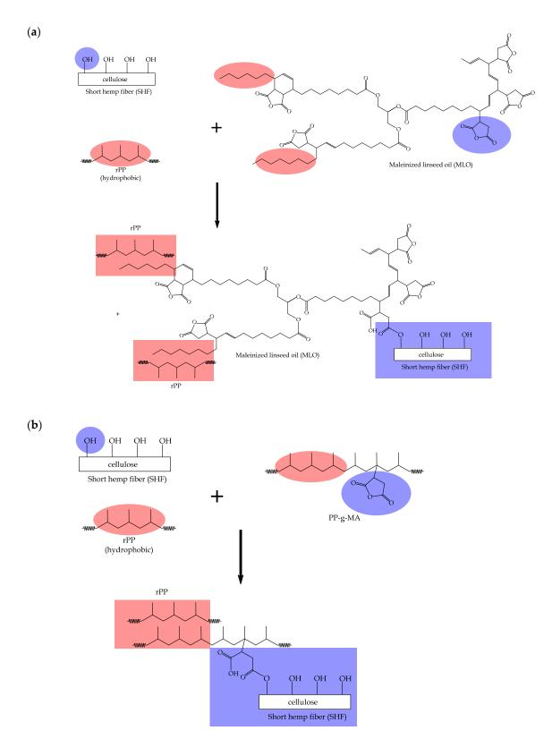
**Scheme 1.** Schematic representation of compatibilization strategies of the rPP/short hemp fiber composites by the utilization of (**a**) maleinized linseed oil (MLO); (**b**) polypropylene graft maleic anhydride (PP-g-MA).
