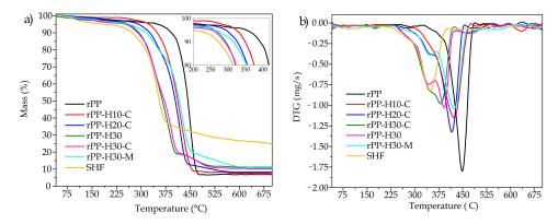
**Figure 4.** Comparative plots of (**a**) thermogravimetric curves and (**b**) DGT curves of the rPP/hemp fiber composites with different compatibilizers.
