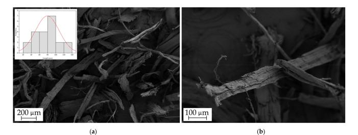
**Figure 1.** FESEM images of short hemp fiber at (**a**)  $50 \times$  with a scale marker of 200 µm with a fiber fineness histogram and (**b**)  $125 \times$  with a scale marker of 100 µm.
