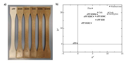
**Figure 7.** (**a**) Injection-molded rPP-SHF composites, (**b**) summary of CIELEAB color space (*L*\*, *a*\*, *b*\*) results of rPP-SHF composites.
