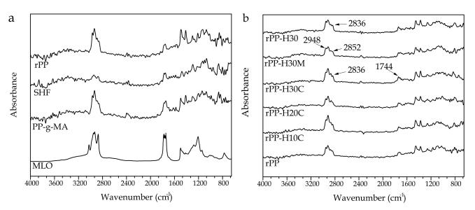
**Figure 8.** (a) Fourier-transform infrared (FTIR) spectra, from bottom to top, of rPP, SHF, PP-g-MA, and MLO; (b) FTIR spectra of the different composites.
