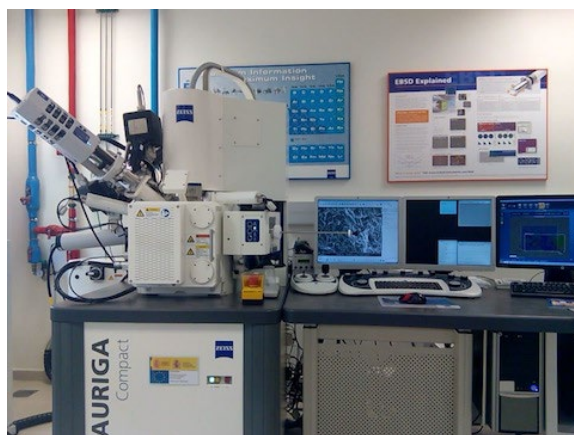
Figure 2.4. FESEM Microscope with attached focalized ion beam (FIB) located at the UPV.
