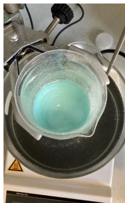
Figure 2.2. Evaporation solution of nickel nitrate, oxalic acid and tin oxalate into a silica bath at 60 °C.
