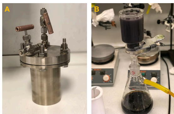
Figure 2.1. Stainless-steel autoclave employed for variable atmosphere hydrothermal synthesis ( A ) and synthesis mixture after hydrothermal treatment under vacuum filtration ( B ).
