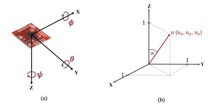
**Figure 4.** (a) The Printed Circuit Board (PCB) axis system in each DOM and yaw ( $\psi$ ), pitch ( $\theta$ ), and roll ( $\phi$ ). (b) The absolute coordinate system for a DU uses a unitary point to locate the relative position of the DOMs of the DU.
