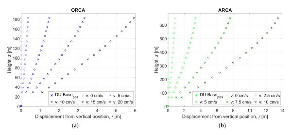
**Figure 5.** Mechanical model (MM) application to line shape in KM3NeT. (**a**) Line shape in ORCA for different sea currents values. (**b**) Line shape in ARCA for different sea current values.
