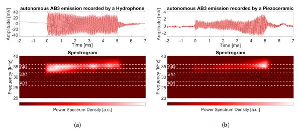
**Figure 3.** Pulse signal received (time scale is relative to detection time) by different DUs. The distinction of the Acoustic Beacon (AB) emitter is clearly observed in the spectrogram. (**a**) The AB pulse recorded by a hydrophone and its spectrogram. (**b**) The AB pulse recorded by a piezoceramic sensor in the lowest DOM (Floor 1 in Figure 1a) and its spectrogram.
