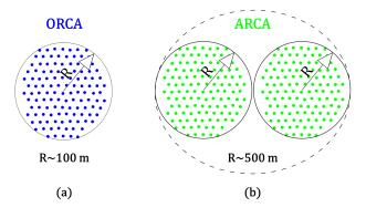
**Figure 2.** Footprint of KM3NeT at the sea bed. (**a**) The block of Oscillation Research with Cosmics in the Abyss (ORCA) has a radius of about 100 m and has 115 DUs. (**b**) ARCA is composed of two blocks of 115 DUs, each with a radius of about 500 m.
