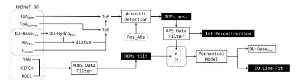
**Figure 7.** DU Line Fit block diagram. This scheme shows the steps in the implementation of the DU Line Fit in KM3NeT detectors.
