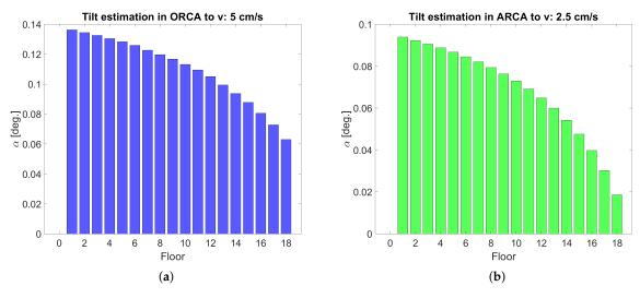
**Figure 6.** Tilt value from MM application for the DOMs in a DU (labeled Floor, with Floor 1 the lowest DOM in the DU) using representative sea current values in ORCA and ARCA. (a) Tilt in ORCA for a typical sea current of 5 cm/s. (b) Tilt in ARCA for a typical sea current of 2.5 cm/s.
