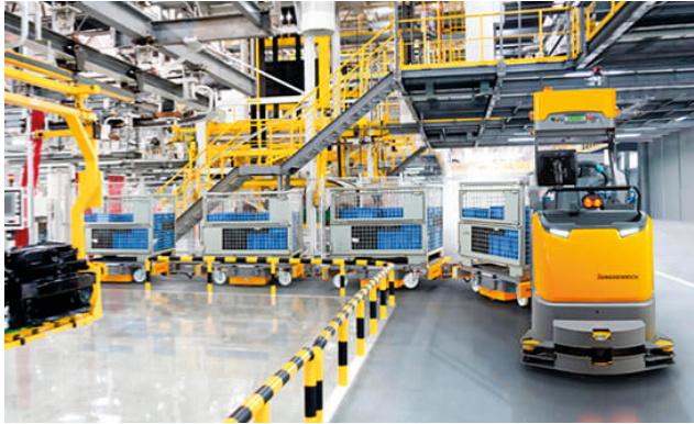
Figura 10.24. Ejemplo de remolque AGV. Extraído de Jungheinrich. (2019). EZS 350a NA Automated Guided Vehicle (AGV) System, Electric Tow Tractor. https://www.logisnextamericas.com/-/media/logisnext/sites/public/images/jh/product/class-iii/features/agv-ezs-350-turning-corner.jpg .
