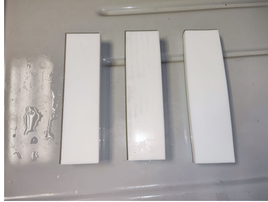
Figure 4.10: Cured PGS in confined volume 72 hours.
