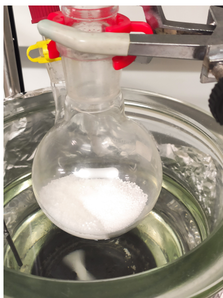
(a) SA and Gly mixed in the flask, getting immersed in the oil.
