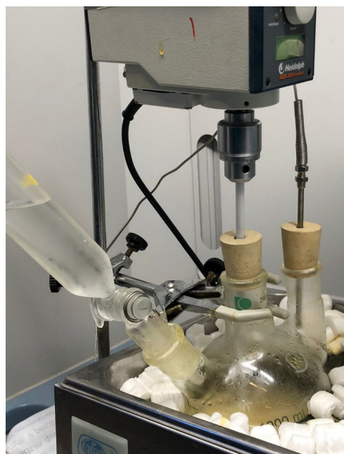
Figure 2. Schematic representation of the epoxidation process of Brazil nut oil.
