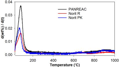
Figure 7. Activated carbon DTG curve.
