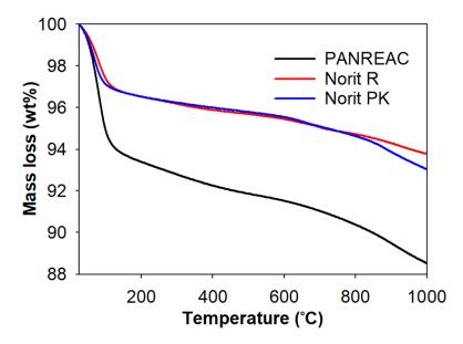
Figure 6. Activated carbon TGA thermal stability curve.
