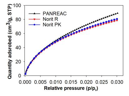
Figure 5. CO<sub>2</sub> adsorption isotherms of the activated carbons measured at 0 °C.
