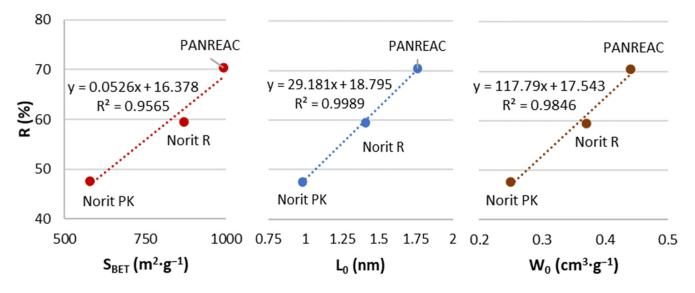
**Figure 8.** Correlations between specific surface area ( $S_{BET}$ ), total micropore volume ( $W_0$ ), and average micropore width ( $L_0$ ) with rejection index (R).
