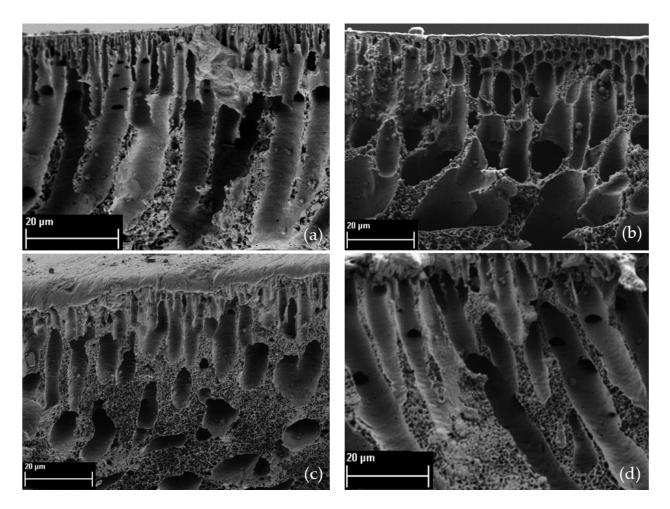
**Figure 13.** FESEM images of the membrane cross-sections of M0 (**a**), M2 (**b**), M4 (**c**), M9 (**d**). Note: M0 (no AC); M2 (PANREAC, 0.50%); M4 (Norit R, 0.50%); M9 (Norit PK, 0.50%).
