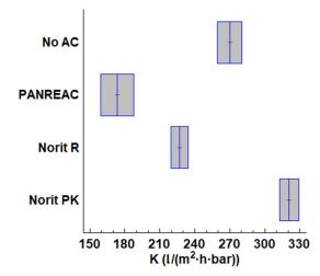
Figure 2. Tukey's diagram for initial membrane permeability for each type of activated carbon added.
