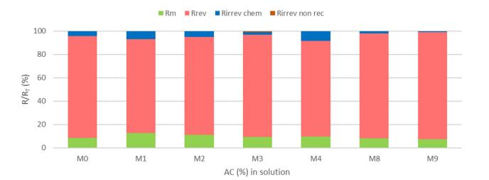
**Figure 9.** Analysis resistance contribution to the total. R<sub>T</sub>, total resistance; R<sub>m</sub>, intrinsic membrane resistance; R<sub>rev</sub>, reversible resistance; R<sub>irrev chem</sub>, chemical irreversible resistance; and R<sub>irrev non rec</sub>, irreversible non-recoverable resistance. Note: M0 (no AC); M1 (PANREAC, 0.10%); M2 (PANREAC, 0.50%); M3 (Norit R, 0.10%); M4 (Norit R, 0.50%); M8 (Norit PK, 0.10%); M9 (Norit PK, 0.50%).
