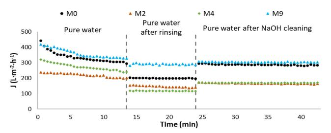
The membrane fluxes from the fouling experiments measured at 1 bar of TMP are presented in Figure 10, reinforcing the results discussed and conclusions made previously. The rinsing and chemical cleaning denote partial or total recovery of the original fluxes.
