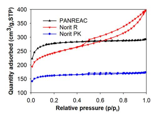
Figure 3. N<sub>2</sub> adsorption–desorption isotherms of the activated carbons measured at -196 °C.
