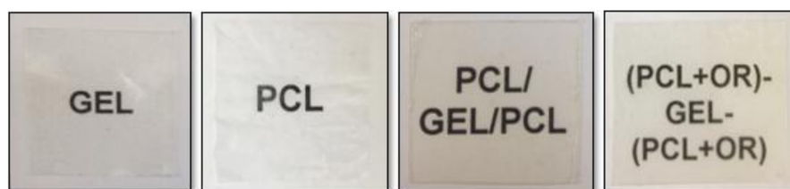
Figure 4. Contact transparency pictures, from left to right, GEL, PCL, PCL-GEL-PCL, and (PCL+OR)-GEL-(PCL+OR) films.
