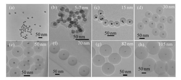
**Figure 1.** TEM images of silica encapsulated gold nanoparticles. Different silica shell thicknesses were produced by MAS when concentration of TEOS raised from none (**a**), 1 mM (**b**), 2 mM (**c**), 3 mM (**d**), 5 mM (**e**), 10 mM (**f**), 15 mM (**g**), up to 20 mM (**h**). Reproduced with permission from [84]. Elsevier, 2011.
