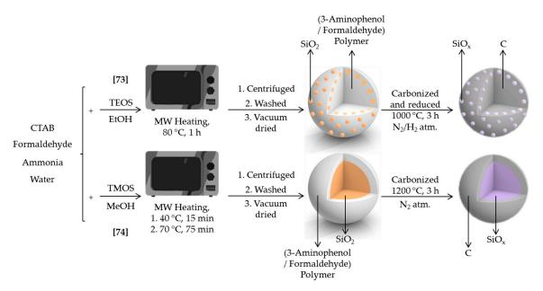
**Scheme 4.** Synthesis scheme for the microwave assisted synthesis of  $C/SiO_x$  nanocomposite [73] and  $SiO_x@C$  [74].
