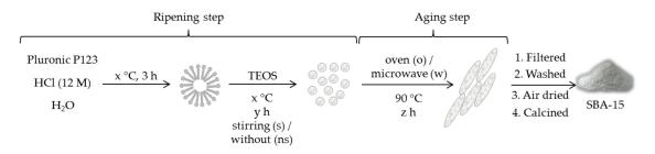
**Scheme 3.** General synthesis scheme for the preparation of SBA-15 [64]. Different ripening temperatures (x = 28, 40 or 55 °C), ripening times (y = from 2 to 24 h), stirred/unstirred samples (s/ns), aging times (z = from 2 to 24 h), and oven/microwave (o/w) conditions were tried. Optimal conditions were found to be x = 40 °C, y = 2 h, stirring (s), and microwave for z = 2 h.
