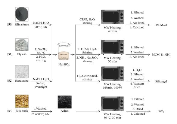
**Scheme 2.** Synthesis scheme for the microwave assisted synthesis of silica materials [50–53] by using non-conventional silicon sources.
