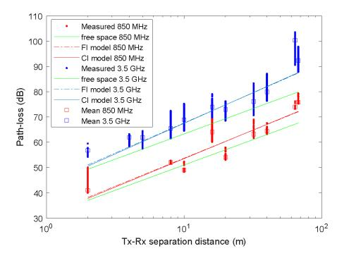
**Figure 5.** Measured path loss, predicted path loss using the FI and CI models, and mean path loss at 850 MHz and 3.5 GHz.
