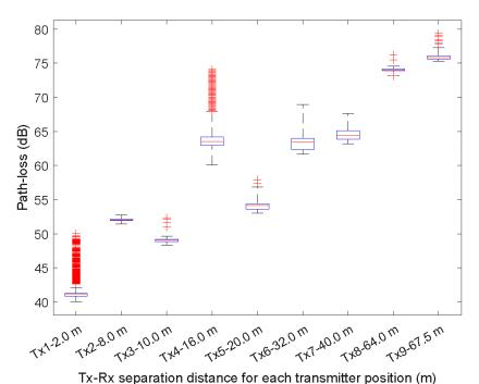
**Figure 6.** Box plots of the path loss as a function of the Tx-Rx separation distance at 850 MHz.
