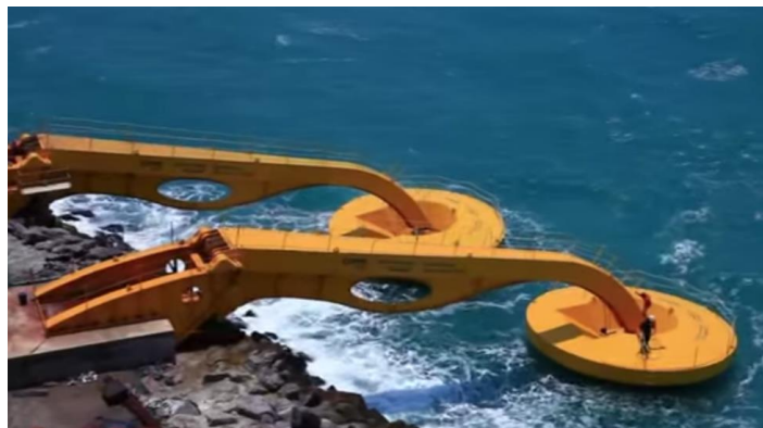
Figure 4. Seahorse power take off system, Brazil Pecem [25].
