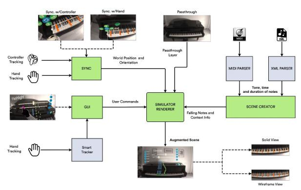
FIGURE 2. Architecture of the application.
