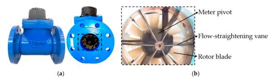
**Figure 3.** Cross-section and longitudinal views of Woltman meter (**a**); detail of the internal part of the horizontal-axis Woltman meter with the meter pivot and six flow-straightening vanes (**b**).
