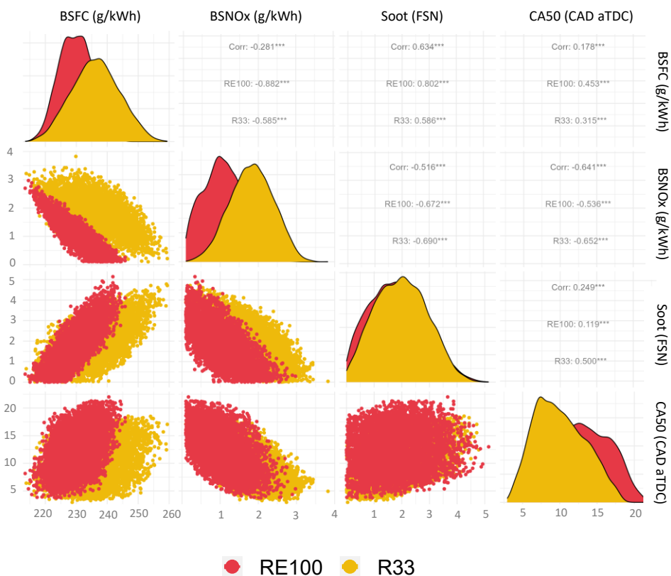
Figure 4. Correlation matrix of the optimization space for the BSFC, BSNO x , Soot and CA50 for the R33 and RE100 fuels at the operating condition 2000 rpm @ 8 bar. Significant values are represented as *p<0.05, **p < 0.01, ***p<0.001.
