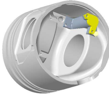
Figure 3.15: Piston with installed battery case.
