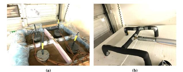
Figure 5-7: The four-column test setup: (a) Four separated columns filled with sand and saturated with water, and (b) Connection of the grout columns to the circulation pump.
