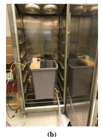
Figure 5-1: The single-column test rig: (a) The sandbox, cooling chamber, and data acquisition system, and (b) Water tank with a mounted heating system inside the cooling chamber.
