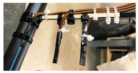
Figure 5-5: Thermocouples with waterproof covers and a wiring system were fixed in position along with a wooden stick.
