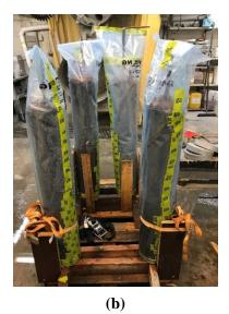
Figure 5-3: Casting and curing of the grout columns: (a) Filling the grout through the funnel, and (b) Curing the grout columns.
